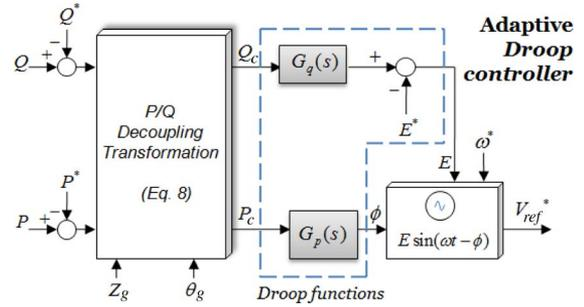
Fig. 5. Block diagram of the adaptive droop control.
