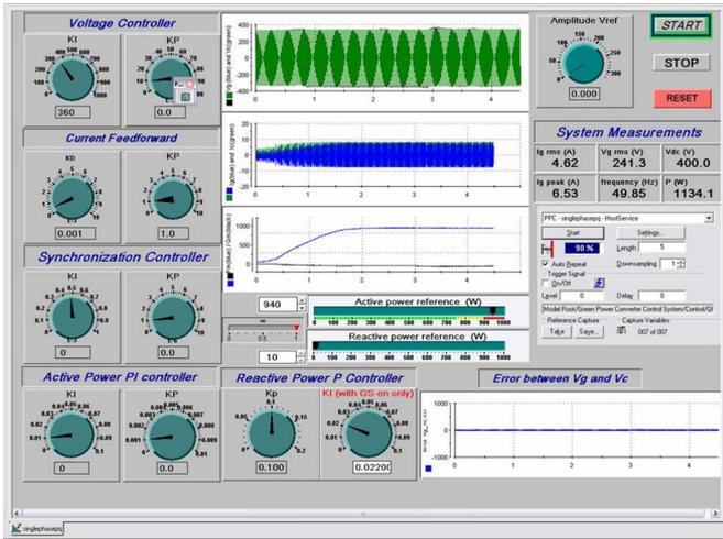
Fig. 17. Panel supervisor of the ControlDesk from dSPACE.
