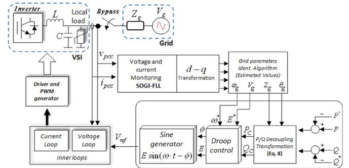
Fig. 9. Block diagram of the SOGI and proposed adaptive droop control with grid-connected to autonomous mode transition capability.
