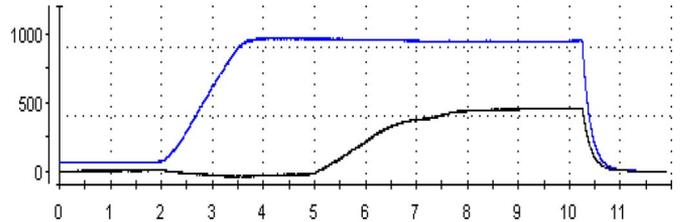
Fig. 21. Transition from islanding to grid-connected mode: (a) Synchronization process (grid and VSI voltages) and (b)  $P$  and  $Q$  for  $t > 2$  s in islanding mode and  $t > 2$  s in grid-connected mode. In  $t = 5$  s,  $P$  changes from 0 to 1000 W, in  $t = 10$  s,  $Q$  changes from 0 to 500 var, and in  $t = 11$  s, the system is disconnected. (Blue line)  $P$  and (black line)  $Q$ .
