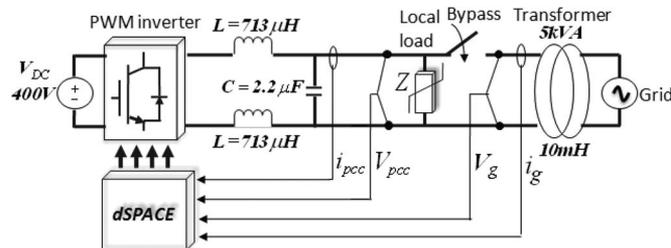
Fig. 16. Scheme of the experimental setup.
