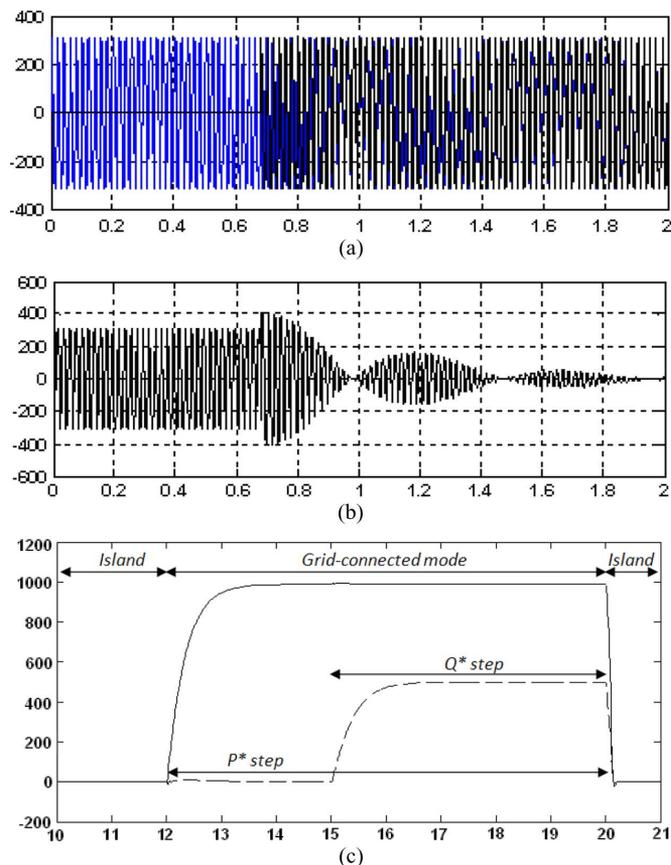
Fig. 15. Transition from islanding to grid-connected mode. (a) Synchronization process (grid and VSI voltages). (b) Error between grid and inverter voltages. (c)  $P$  and  $Q$  for  $t < 12 \text{ s}$  in islanding mode and  $t > 12 \text{ s}$  in grid-connected mode. In  $t = 17 \text{ s}$ ,  $P$  changes from 0 to 1000 W, in  $t = 19 \text{ s}$ ,  $Q$  changes from 0 to 500 var, and in  $t = 20 \text{ s}$ , the system is disconnected from the grid.
