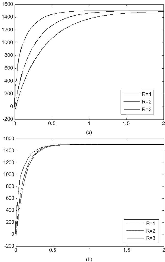
Fig. 14. Start-up of  $P$  for different line impedances (a) without and (b) with the estimation algorithm of  $Z_g$ .
