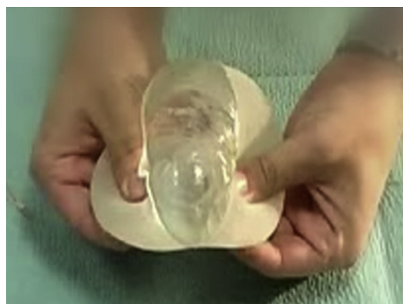
Figure 1 Image of cohesive 'form-stable' silicone implant demonstrating the difficulty in forcing the gel out of the elastomer even when completely disrupted.
