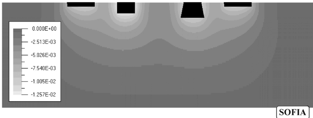
Fig. 9. Vertical movements in subsoil (mm)—pre-remedial work.
