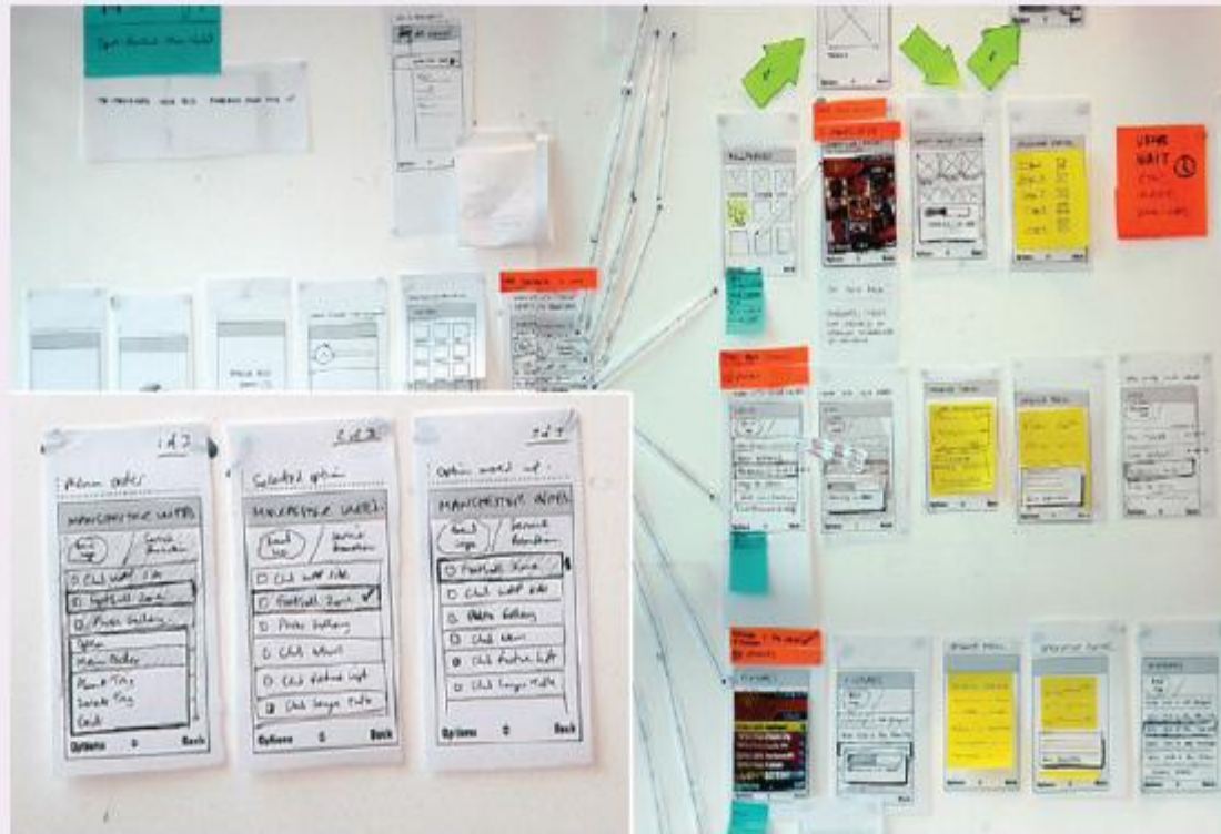
Figure 11.6 Prototype developed for cell phone user interface
