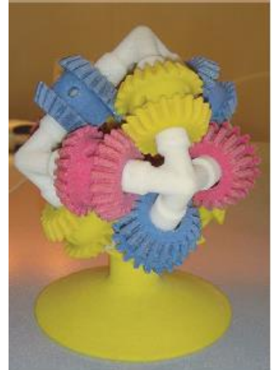
Figure 11.1 (a) Color output from a 3D printer: all the gears and rods in this model were 'printed' in one pass from bottom to top, and when one gear is turned, the others turn too.
