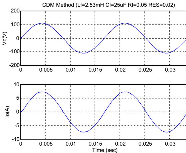
Fig. 10. Output voltage and current waveforms with L-C filter designed by CDM (Mode II).
