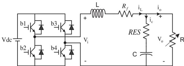
Fig. 1. Circuit of single phase PWM-VSI inverter.
