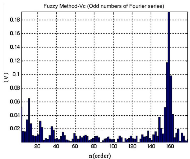
Fig. 23. Harmonic spectrum of output voltage for FLC (Mode II).
