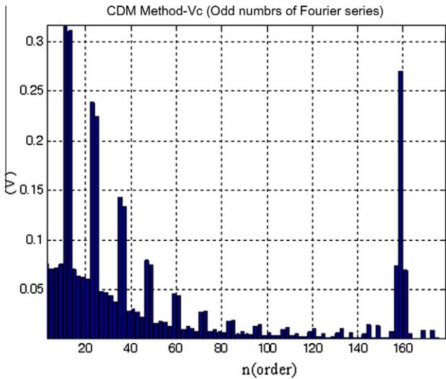
Fig. 17. Harmonic spectrum of output voltage for CDM (Mode II).
