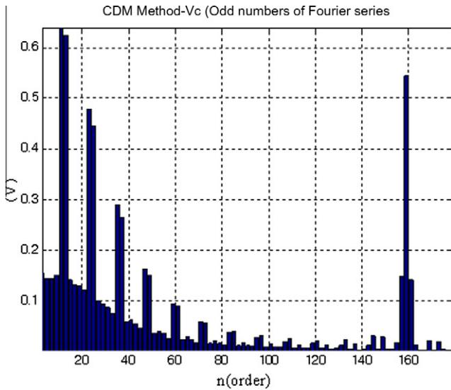
Fig. 19. Harmonic spectrum of output voltage for CDM (Mode III).
