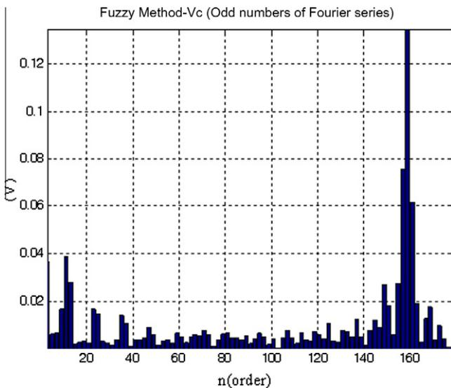
Fig. 21. Harmonic spectrum of output voltage for FLC (Mode I).
