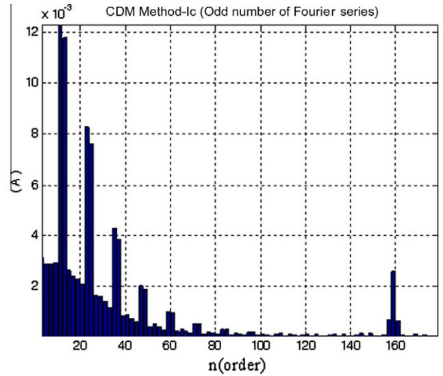
Fig. 16. Harmonic spectrum of output current for CDM (Mode I).
