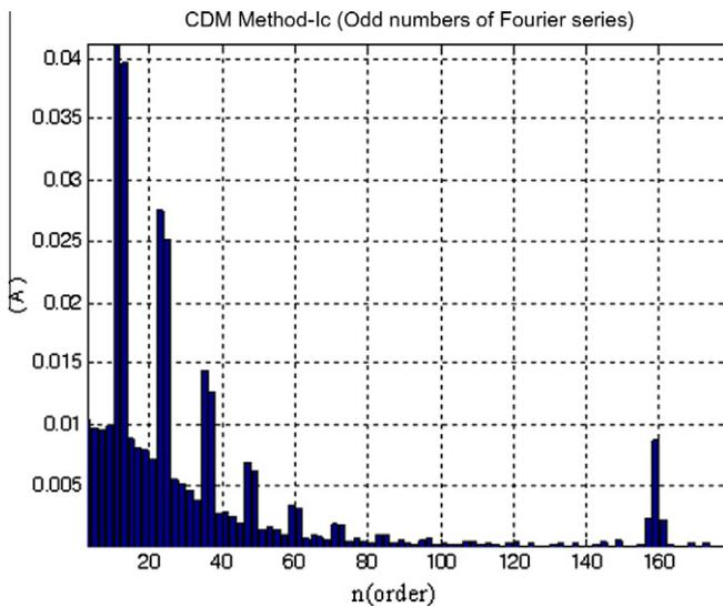
Fig. 20. Harmonic spectrum of output current for CDM (Mode III).
