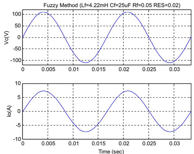
Fig. 12. Output voltage and current waveforms with L-C filter designed by FLC (Mode I).
