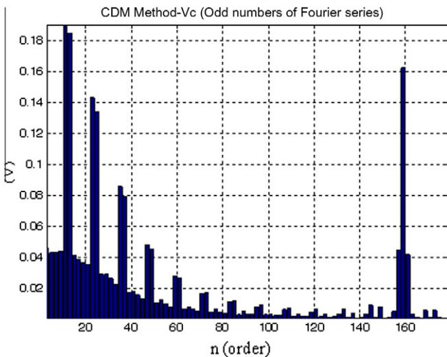
Fig. 15. Harmonic spectrum of output voltage for CDM (Mode I).
