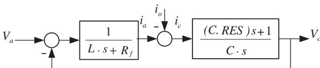
Fig. 2. Equivalent block diagram of L-C filter for single phase inverter.
