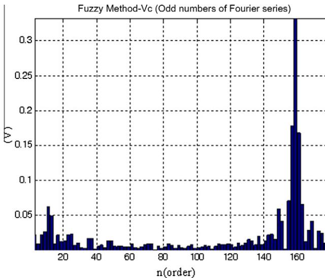
Fig. 25. Harmonic spectrum of output voltage for FLC (Mode III).
