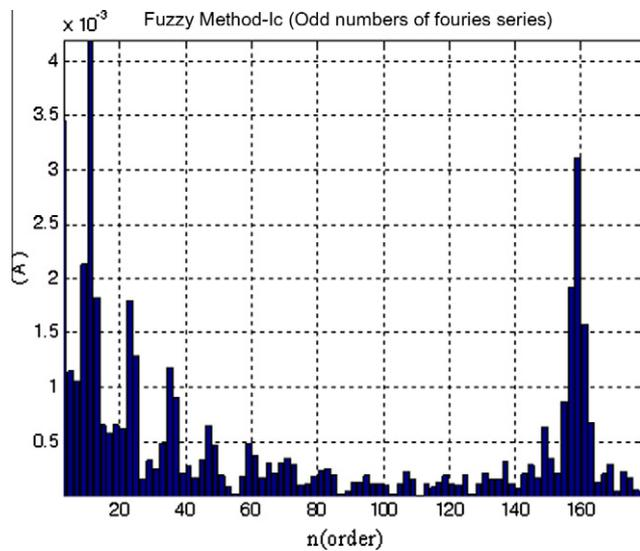
Fig. 24. Harmonic spectrum of output current for FLC (Modell).
