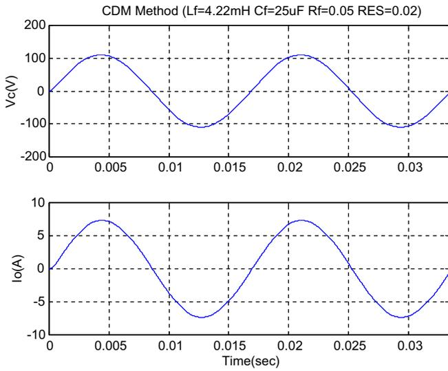
Fig. 9. Output voltage and current waveforms with L-C filter designed by CDM (Mode I).
