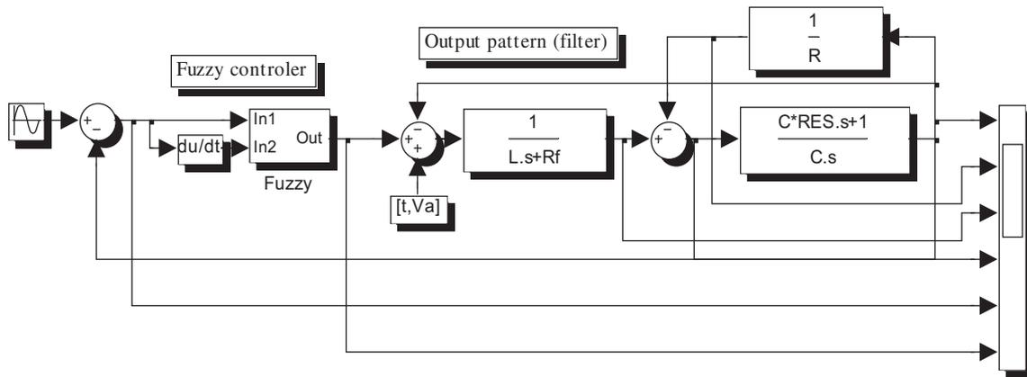
**Fig. 8.** Matlab-Simulink structure for FLC.
