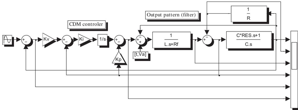
**Fig. 7.** Matlab-Simulink structure for CDM.
