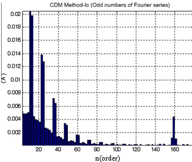
Fig. 18. Harmonic spectrum of output current for CDM (Mode II).
