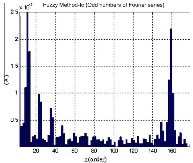
Fig. 22. Harmonic spectrum of output current for FLC (Mode I).
