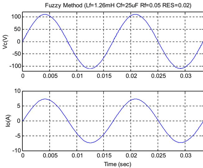
Fig. 14. Output voltage and current waveforms with L-C filter designed by FLC (Mode III).
