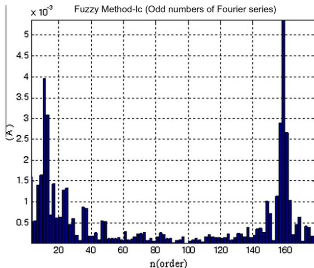
Fig. 26. Harmonic spectrum of output current for FLC (Mode III).
