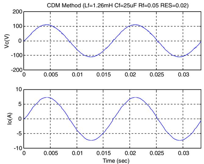
Fig. 11. Output voltage and current waveforms with L-C filter designed by CDM (Mode III).
