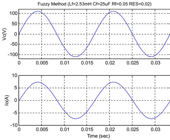
Fig. 13. Output voltage and current waveforms with L-C filter designed by FLC (Mode II).
